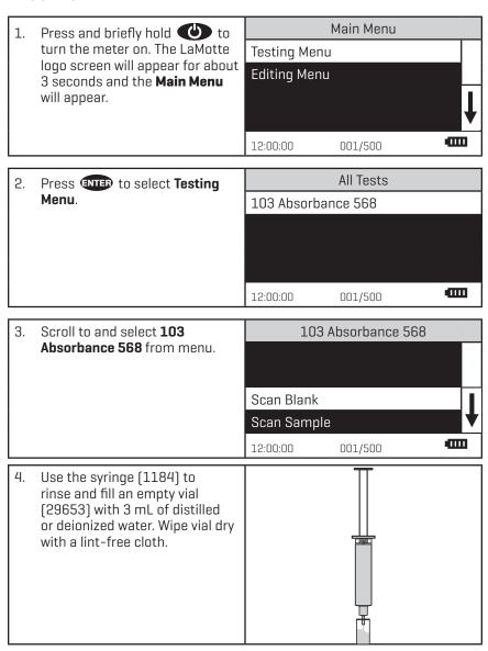
5. Insert vial into chamber, close lid and select Scan Blank. Use the syringe (1184) to rinse and fill the same vial with 3 mL of standard solution. Wipe vial dry with a lint-free cloth. Insert vial into chamber. Close 103 Absorbance 568 lid. Select **Scan Sample**. Record 1.350 result. Scan BLank Scan Sample 1111 12:00:00 001/500 103 Absorbance 568 Press V to scroll to 8. Calibrate. 1.350 ppm
